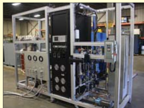
A major manufacturer had a requirement for an integrated control system that required the design and assembly of a structural aluminum machine frame, pneumatic and automation assemblies, hose and stainless steel fittings and a PLC driven control system.
