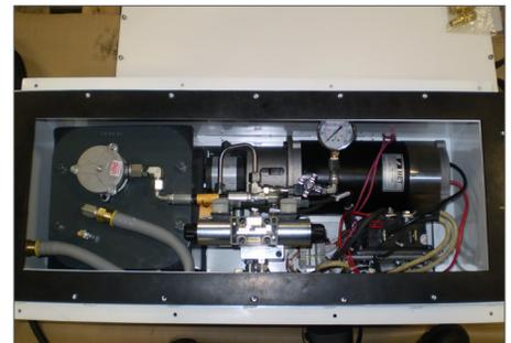
*Hydraulic power units were custom designed and built by Sorensen Systems to provide load leveling to assist in loading vehicles on aircraft.*
