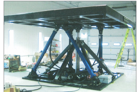
The hydraulically actuated motion platform capable of carrying a 30,000 pound payload was originally designed and manufactured to test shipboard equipment.
